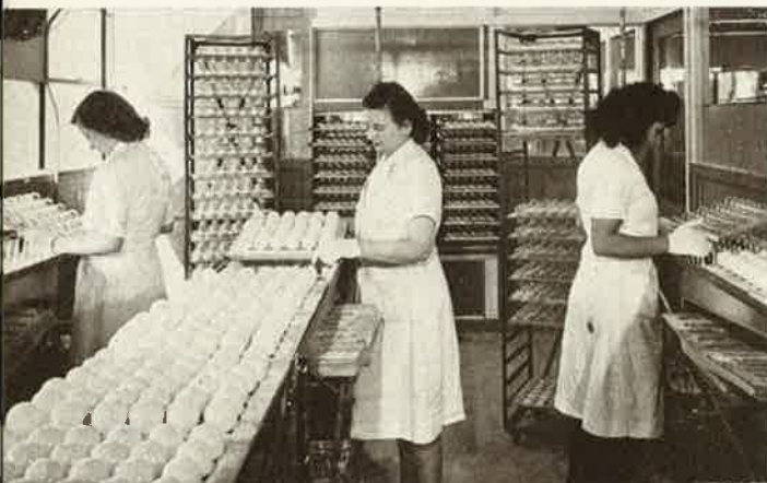
COATING AND DRYING is done by putting bulbs over spigots (at left) that squirt coating inside, then sending them into drying tunnel. Operators L to R: Elizabeth Stewart, Barbara Doty, Carmella Bellino.
